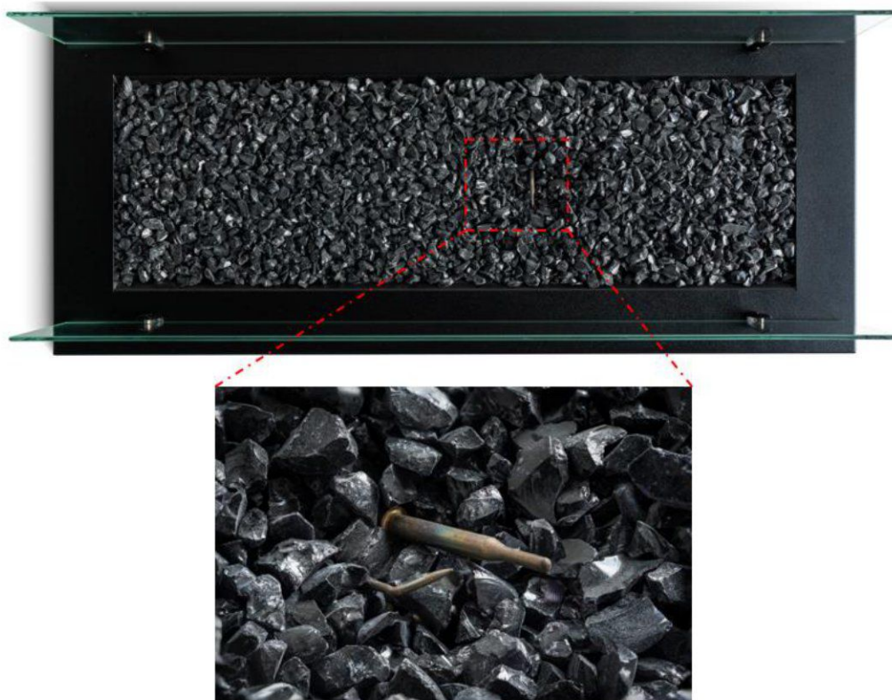
Fig. 2 – RIO top view and ignition elements detail
